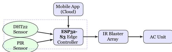
Figure 1. AeroSense Functional Block Diagram.
